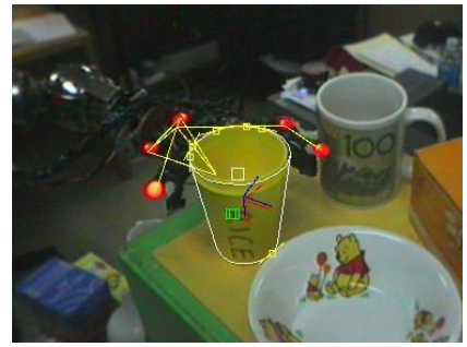
(c) Visual servoing to planned grasp.
